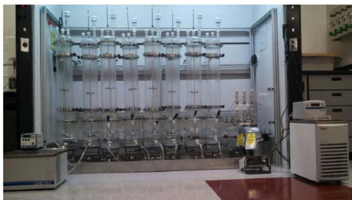
Figure 5: Transparent glass column vapor space corrosion test apparatus proposed by Fuentes et al. (reproduced from [29] – © NACE International 2015)
