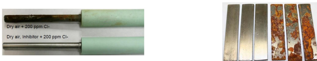
Figure 3: Electrical resistance (left) and weight loss (right) specimens proposed by Bavarian et al. (reproduced from [28] – © NACE International 2016)
