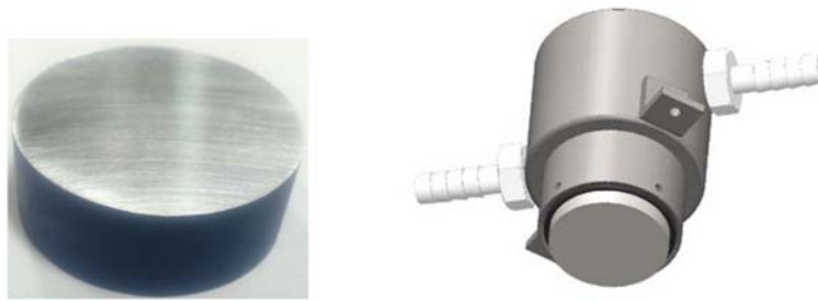
Figure 15: (a) picture of a carbon steel WL sample, (b) WL sample mounted in the cooling/heating system.
